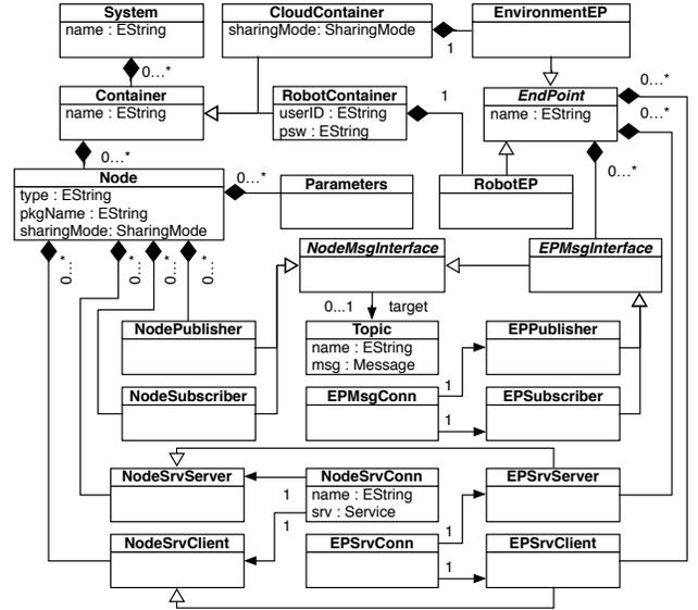
Fig. 2: Rapyuta’s component meta-model
